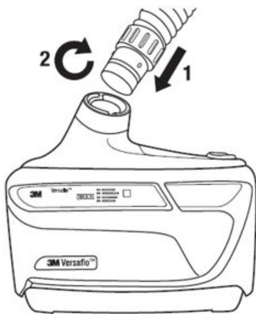
**Figure 7: Removing breathing tube**
